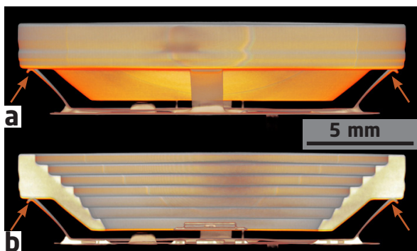
Overlaid volume rendering of the operating (grey) and turned off (orange) LED sandwich, a) from the outside and b) cut in the center.
