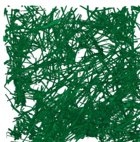
3D-rendering of the fiber structure of stone wool
