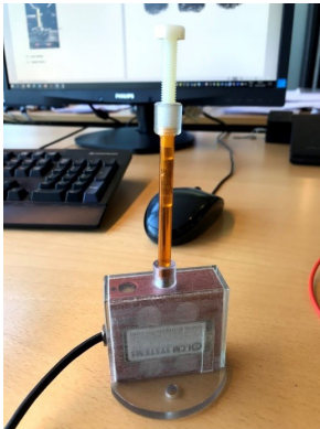
Photograph of the in situ cell. The white screw on top compresses the sample which is kept in the orange tube. The compression cell to measure the load is placed beneath the tube.
